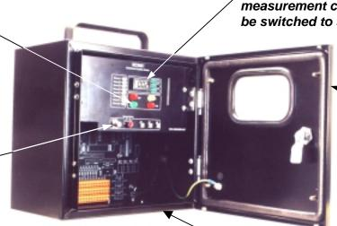
Digital display scans through measurement channels and can be switched to show alarm levels
