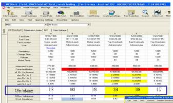
Trend Phase-to Phase resistance over time. If an out of tolerance condition occurs MCEGold will alert you.
