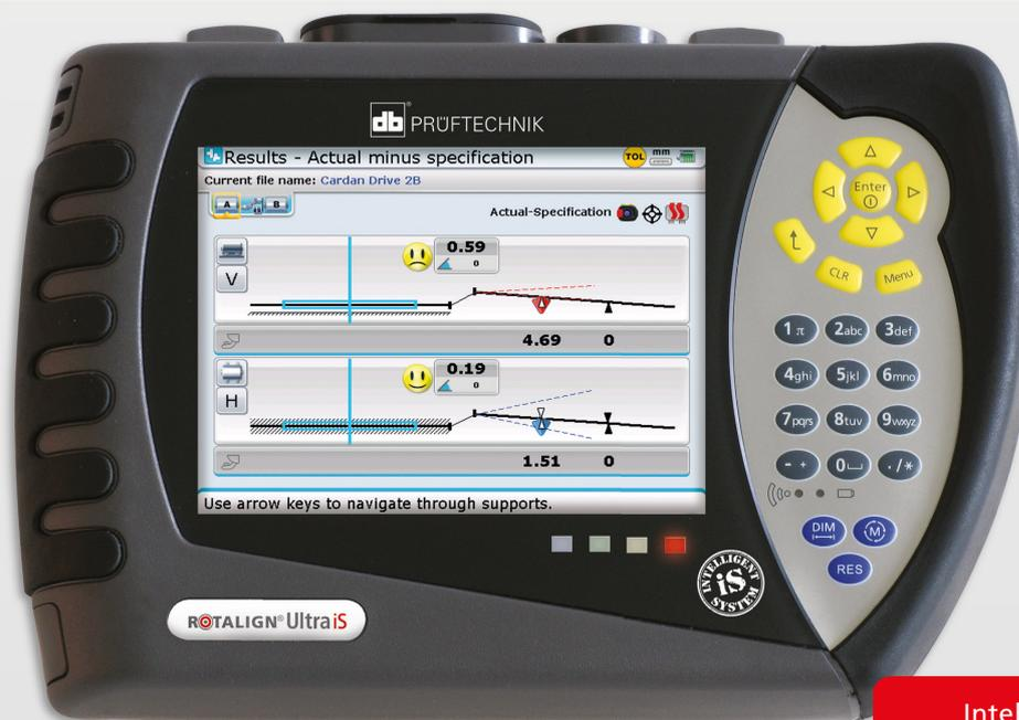
In the Result screen the cardan angle and foot position are displayed as well as the tolerance status through a 'Smiley'.
