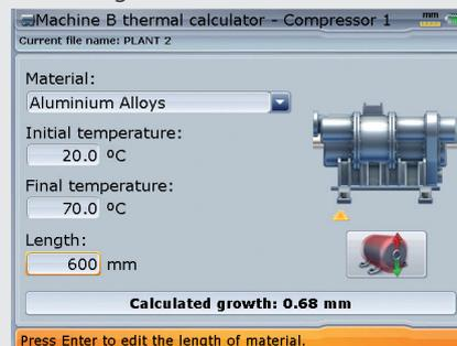
Used to determine the machine expansion parameters mathematically.
