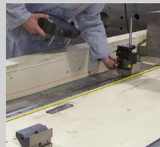
Measurement of vertical and horizontal straightness in response to industry demands
