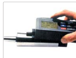
Extra start button easy accessible for hand-held operation
