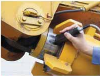
● Diagnosing wear and tear using hardness measurements
