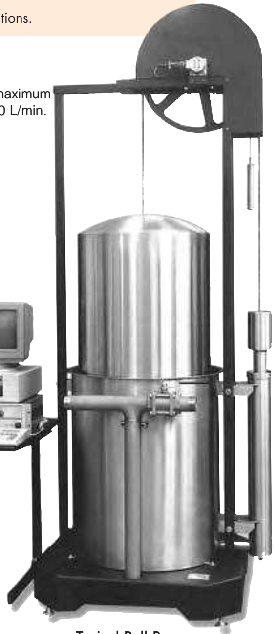
Typical Bell Prover used for NIST traceable calibrations
