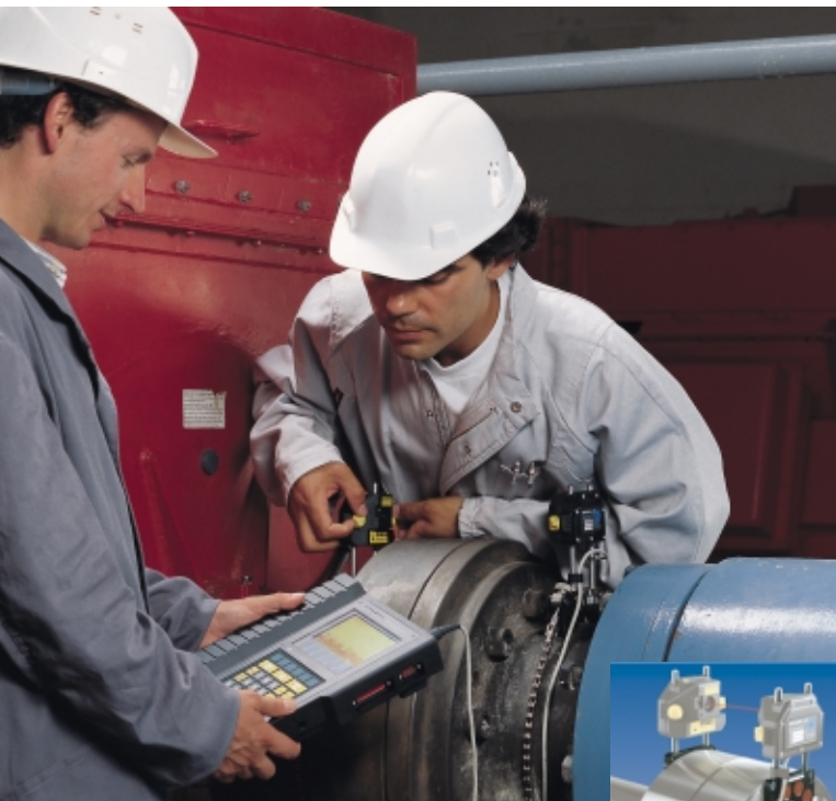
A range of brackets for all types of machines and couplings ensure fast alignment results.
