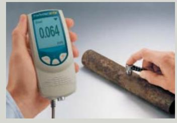
**UTG Std** measures the remaining wall thickness of steel, cast iron and more due to the effects of corrosion and erosion.
