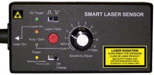
Smart Laser Sensor is an internal battery-powered optical speed sensor utilizing a visible Class 3R Laser for a TTL pulse output. Operating range up to 65 feet (19.8 m) with reflective tape and up to 3 feet\* (1 m) from contrasting color targets, keyways, bolt heads or blades.
