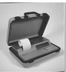
displayed during the calibration runs. The display indicates when to start and stop the rotor and when to add or remove the trial weights. The balance corrections are instantly computed and shown in direct weight units.
