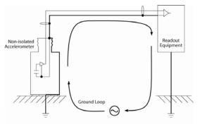
Figure 3. Ground Loop From Improper Grounding
