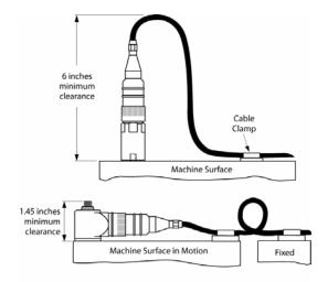
Figure 5. Cable Anchoring
