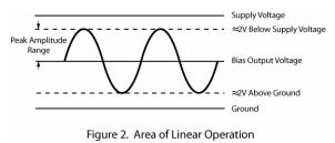
the output of the sensor. The output voltage swing determines the peak vibration amplitude range. (See figure 2.) Thus an accelerometer with a sensitivity of 100 mV/g, and a peak output swing of 5 volts, will have an amplitude range of 50 g peak.
