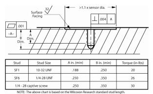
Figure 7. Stud Mounting: Surface Preparation
