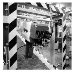
The On-line JE series are used in the ferrite drying process to measure the moisture content at the entrance and exit of a dryer.
