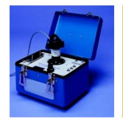
Three shakers to choose from! All three shakers are battery powered, portable and have a built-in reference accelerometer and indicator with calibration traceable to the National Institute of Standards and Technology (NIST). The shakers are designed to be used in the field or shop to verify the performance of vibration transducers, connectors, cabling, instruments or permanently installed machine vibration condition monitoring systems or indicators.
