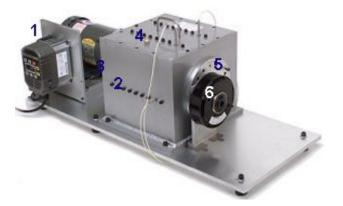
**1.** The gearbox is driven by a 3 hp. induction motor with inverter speed control for an input speed range of 0 to 4,000 rpm. The inverter can be programmed for higher speeds, but care must be exercised to assure proper lubrication and temperature control. The inverter is initially programmed to permit simple start/stop and scrolling to different speeds measured in hertz (revolutions per second); however, it may also be set up to permit PLC control.
