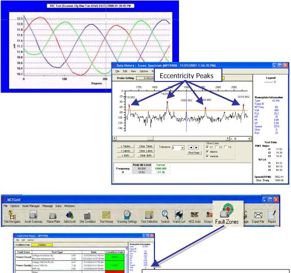
The MCEMAX powered by MCEGold<sup>™</sup> provides a Fault Zone Report, which is a one-page summary of the test results relevant to the six fault zones. The Fault Zone Report may be reached directly through the Fault Zones icon on the toolbar.
