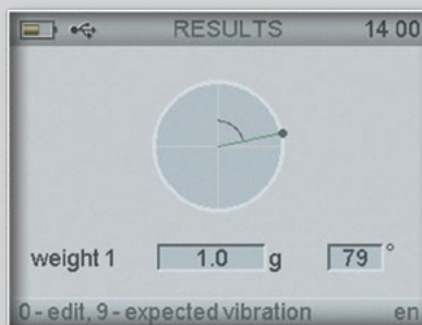
Calculation of balancing mass location
