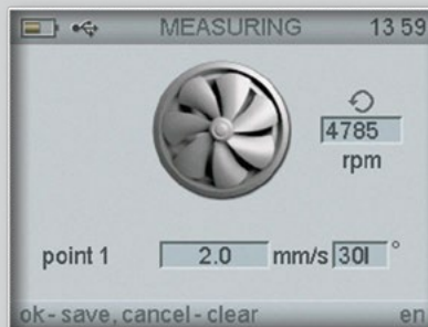
Vibration and phase measurement
