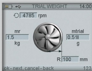
Test weight calculation and installation
