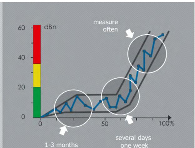
Shock pulse strength depends on a shock velocity  $V$ , if  $A$  represents a shock pulse peak value, then there is a relation of  $A = f(V)$ , while the shock velocity  $V$  also depends on a bearing size, rotation speed and defect size.
