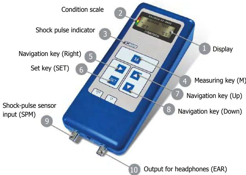
The bearing condition is estimated according to the color condition scale:
