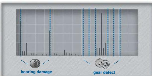
The bearing vibration monitoring allows detecting irregularities in equipment, and to define the reason of such irregularities the spectral vibration diagnostics should be used.
