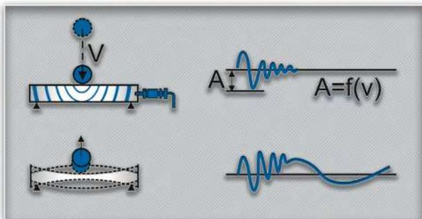
The shock pulse method can be illustrated by the example of a metal ball fall on a metal object. The shock waves will appear in both objects. The shock pulse amplitude is equal to the impact velocity function.
