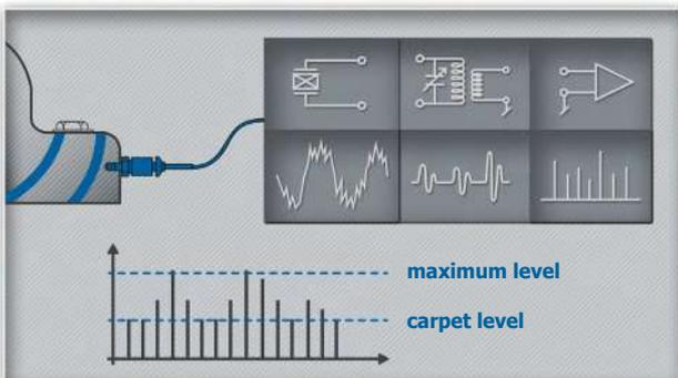
Total shock pulse intensity increases with decreasing of lubrication film thickness. Pronounced shock pulse peaks indicate bearing defects.
