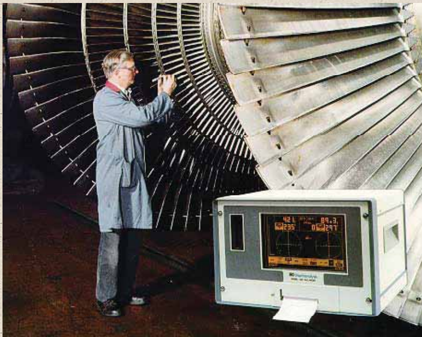
Series 290 - the "brain" of the B140. Precision low speed balancer.
