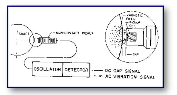
Monitoring the bearing of Turbine in sequent, Compressor, Gearbox, Pump with Journal/Plane Bearings to analyze Shaft Roundness, Shaft Run-Out, Unbalance, Misalignment, Shaft Centerline, Rubbing, Looseness and etc.
