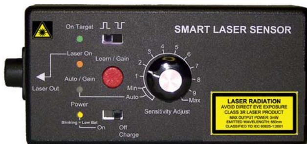
**Smart Laser Sensor** is an internal battery-powered optical speed sensor utilizing a visible Class 3R Laser for a TTL pulse output. Operating range up to 65 feet (19.8 m) with reflective tape and up to 3 feet\* (1 m) from contrasting color targets, keyways, bolt heads or blades.
