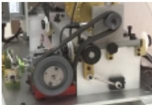
Belt tension can be controlled with an idler lever or by sliding the gearbox. The system can be operated with one or two belts, and the belts can be mismatched. Parallel and angular belt misalignment can be easily introduced to study the effects on vibration signatures.
