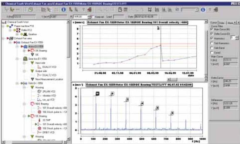
The OMNITREND® PC software provides many options for the display, analysis and ISO-conform documentation and archiving of the measured machine data. Measurement and alarm settings are simple to program with a click of the mouse.
