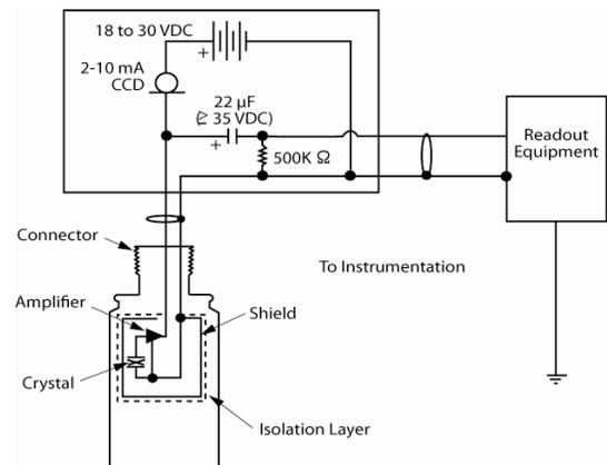
Figure 1. Powering Schematic
