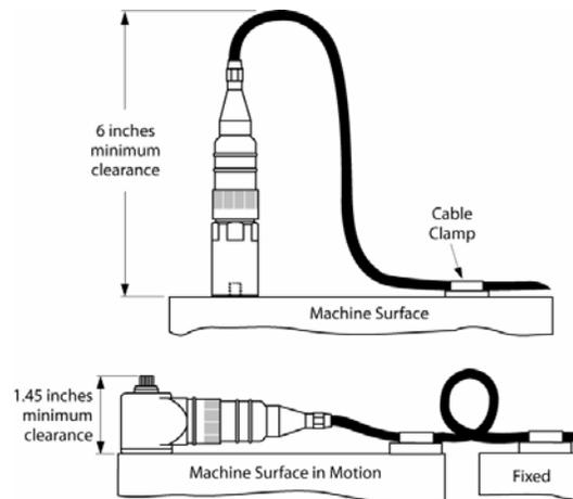
Figure 5. Cable Anchoring
