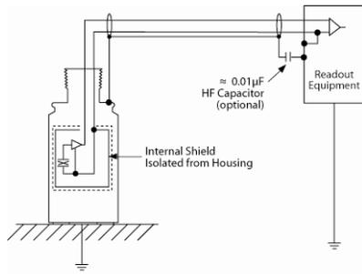
Figure 4. Multiconductor/Shield Configuration
