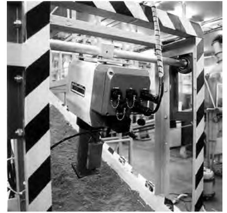
The On-line JE series are used in the ferrite drying process to measure the moisture content at the entrance and exit of a dryer.
