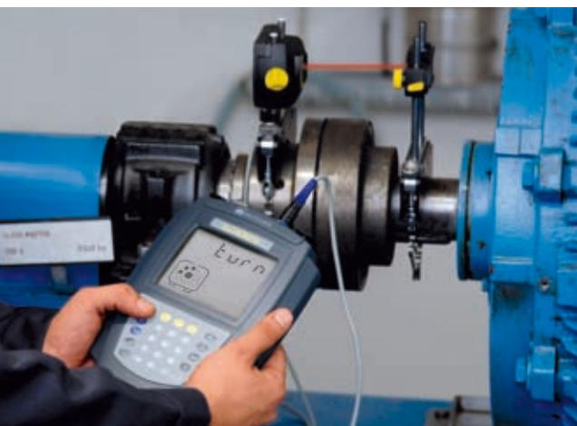
ALIGNEO® merges **precision alignment** with **timesaving comfort** of an innovative laser alignment system.
