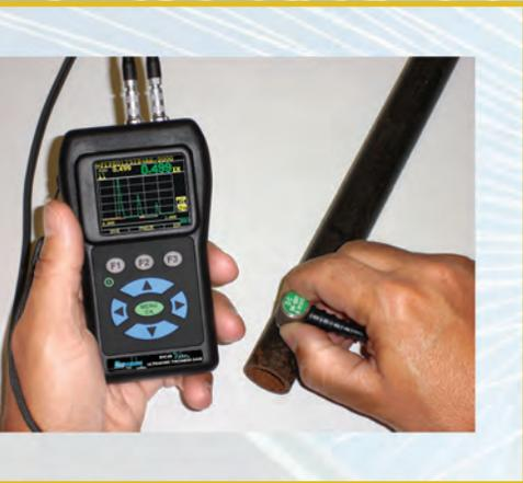
Danatronics is proud to introduce the world's smallest ultrasonic thickness gage with high resolution **COLOR** waveform display, The EHC-09 Wave. Unique features include live **COLOR** A-Scan, B-Scan, 50K thickness reading (5000 waveforms) datalogger with interface program, vibration and **COLOR** change of waveform on alarm.
