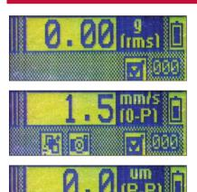
For those precision machines that have very low vibration levels, a precision reading is necessary. In addition to an extra quiet accelerometer that is supplied as a standard accessory, both vPod and vPod II incorporate a built-in gain circuit to amplify small vibration signals and show the reading in precision mode when you turn the gain mode on. This one button gain function allows the user to increase precision by one decimal place.
